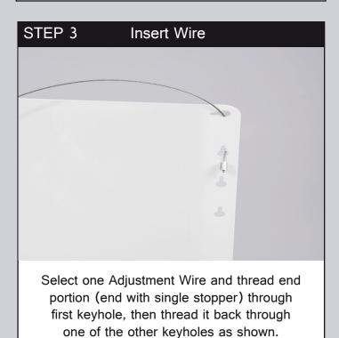
This action locates the wire and presets the reflectors width.
