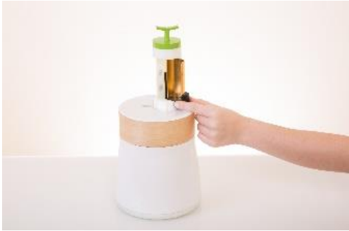
Figure 24: Sliding the Reflector into Sample Drawer
