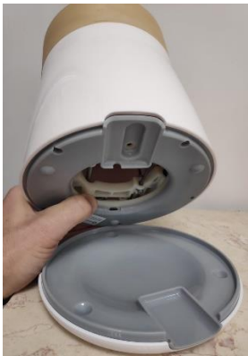
Figure 6: Pulling the Base Off the Device
