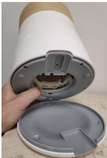
Figure 46: Pulling the Base Off the Device
