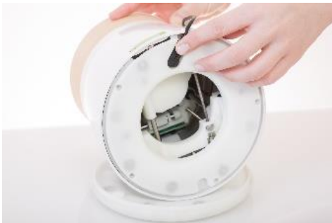
Figure 7: Plugging the Power Supply Cable into the Socket
